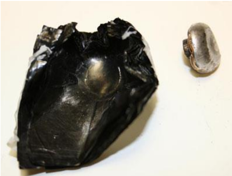
Figure 5.4 CNT fabric stopped a 9MM, jacketed round in controlled ballistics testing. This material shown is roughly the same thickness as six stacked business cards.*
